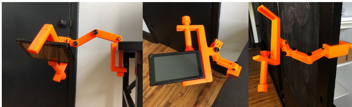
Figure 1) The final 3D printed ASCAP mount
